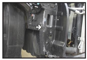
11. Using a reciprocating saw, trim the lip off the face of the frame as shown for baseplate clearance. Do this on both sides of the vehicle. Reinstall the bumper with the existing bolts.
