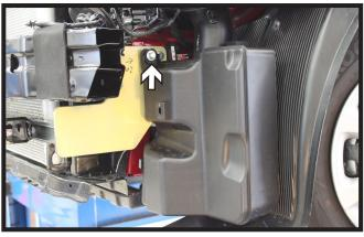
17. Trimming of the air baffle is required before reinstallation. With a utility knife, trim the lower tab off of the air baffle as shown. Remove the 6MM bolt and washer from the baseplate. Reinstall the baffle, using the existing bolts and reinstalling the 6MM bolt and washer into the baseplate.
