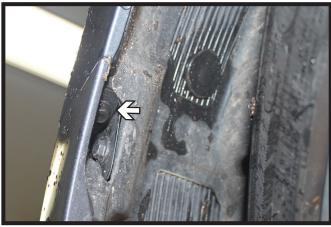
2. In wheel well, using a 10MM socket, remove upper screw from the fascia joint. Do this to both sides of the vehicle.
