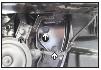
7. Using a 12MM socket, remove the two (2) bolts from bottom of bumper (white). Using a 10MM socket, remove the horn bracket bolt (gray). Do this to both sides of the vehicle. Set the bumper aside.
