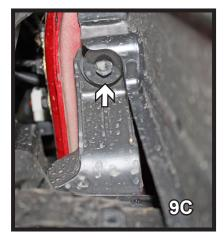
9. On the driver side, remove the push pin (9A - gray). Using a 10MM socket, remove the two (2) screws (9A-white) and the one (1) screw on the underside of the fascia (9C). Disconnect the hose from the air baffle (9B) and remove from the vehicle.
