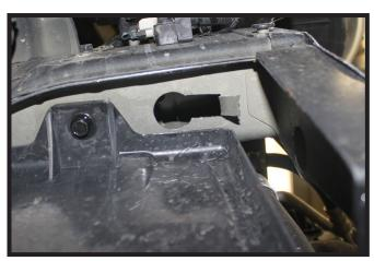
12. Using a reciprocating saw, cut two (2) slits on the bottom hole in the frame and bend the tab out to allow nut plate access. Do this on both sides of the vehicle.
