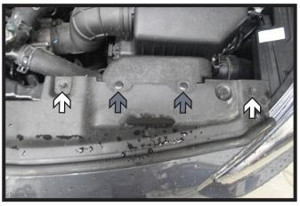
Using a 10MM socket, remove the four (4) screws (white) from the top of the fascia.
