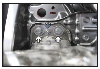
6. Using a 12MM socket, remove the two (2) bolts from top of metal bumper (white). With a 10MM socket, remove the bolt in the backside of the bumper (gray). Do this to both sides of the vehicle.
