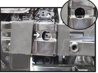
13. On the front of the bumper, toward the outer edge of the bumper, with a 1-1/4" hole saw, cut through the front two (2) layers of the metal bumper for nut plate access. Do this to both sides of the vehicle.
