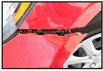
Lift up and pull out the corners of the fascia. Remove the fascia from the vehicle disconnecting any electrical connections and set fascia aside.
