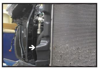
On the passenger side, remove the plastic shrouding next to the radiator for baseplate clearance.
