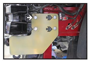
15. Using a 13/32" drill bit, drill top front hole on both sides of the vehicle thru the frame (white). Insure the baseplate remains level. Install 3/8"-16 x 1-1/4" bolts with 3/8" lock and flat washers into the holes and 3/8" nut plates in the frame. Fully tighten all hardware.
