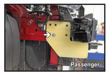
14. Mount the baseplate onto the vehicle using the existing holes on frame rails. On driver side insert a 6MM-1.00 x 45MM bolt into existing hole with 1/4" flat washer. On passenger side, insert a 6MM-1.00 30MM bolt into existing hole with 1/4" flat washer. Level the baseplate and tighten the hardware.
