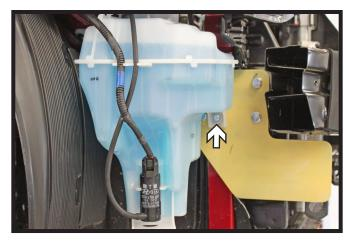
16. Remove the 6MM bolt and washer from the baseplate. Reinstall the washer reservoir, using the existing bolts in the back of the reservoir and reinstalling the 6MM bolt and washer into the baseplate. Reattach all fluid lines and electrical connections.
