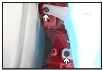
8. Using a Phillips screwdriver, remove the screw at the front of the reservoir (gray). Using a 10MM socket, remove the two (2) screws from the backside of the washer reservoir (white). Disconnect and plug all lines, then set washer reservoir aside.
